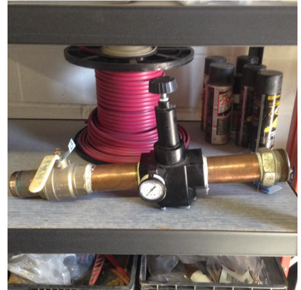
2" Parker 09R813BA with pressure gauge, brass fittings and hose connection ~$850
